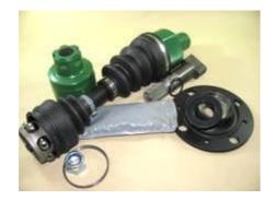
The single-side (set half) contains with: Interconnecting axle with inner tripod joint and outer B-F cv joint, sideplate with bearing, stub axle, seal, seeger circlip, outer joint's boot clamps, grease and nyloc nut.
