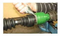
• Fill the joint housing and the cv joint boot with second half of grease.
