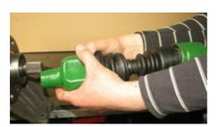
• Install the inner joint of the driveshaft onto the gearbox stub axle, pulling the joint to outside direction. (There is a spring inside the joint).
