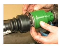
• Install the wire ring into the channel inside the joint housing to keep the ball-cache on place.
